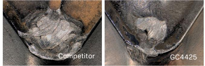
**Result:** The competitor insert has large crater wear, while GC4425 produced 80% more pieces with a stable and predictable flank wear.
