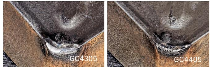
**Result:** Grade GC4405 provided a 130% increase in tool life compared to existing grade GC4305 based on better plastic deformation resistance and crater wear resistance.
