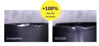
**Result:** Grade GC1205 provided a 100% increase in tool life compared to the competitor thanks to increased flank and crater wear resistance.
